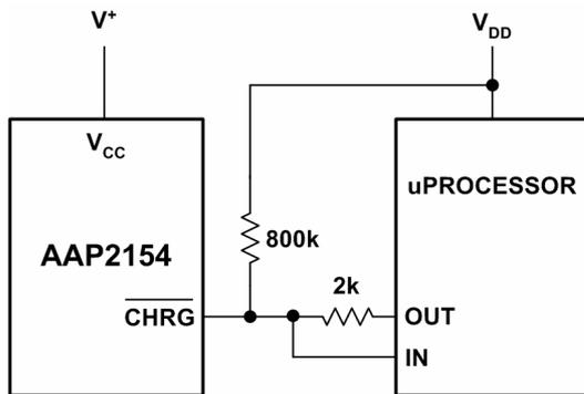
**Figure 10. Using a Microprocessor to Determine CHRG State**
