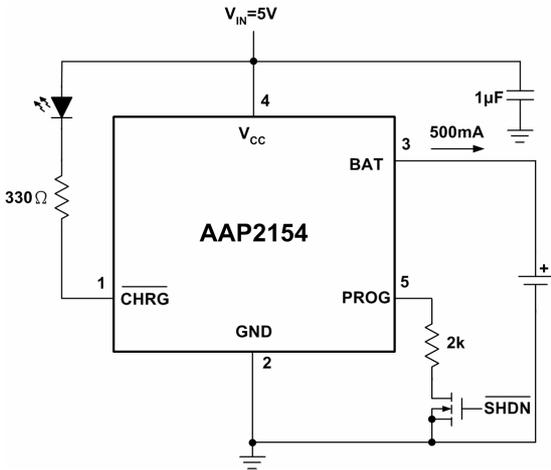
Figure 3. Full Featured Single Cell Li-ion Charger
