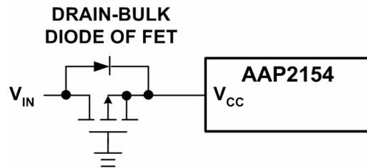
**Figure 11. Low Loss Input Reverse Polarity Protection**
