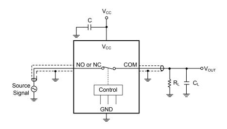
Test Circuit 6. -3dB Bandwidth
