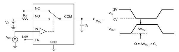
Test Circuit 7. Charge Injection (Q)
