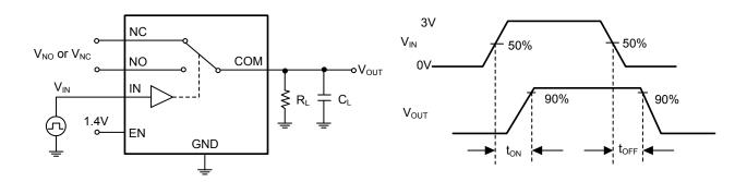
Test Circuit 2. Switching Times ( $t_{\text{ON}}$ ,  $t_{\text{OFF}}$ )
