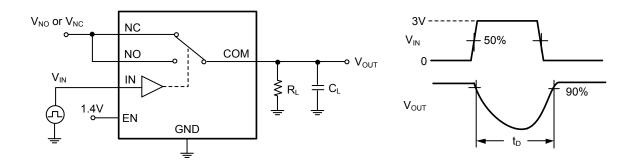
Test Circuit 3. Break-Before-Make Time Delay (t<sub>D</sub>)
