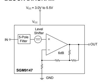
NOTE: Power supply  $V_{\text{CC}}$  must be sequenced on first before input video signals.
