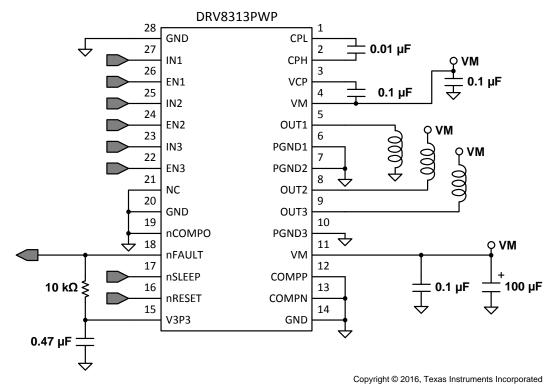
Figure 17. Three Independent Load Connections Schematic
