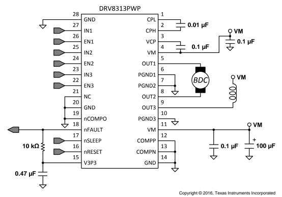
Figure 16. Brushed-DC and Solenoid Schematic
