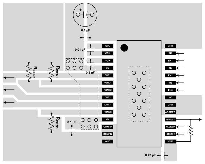
Figure 19. Recommended Layout Example For HTSSOP PWP Package
