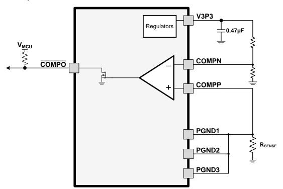
Figure 12. Comparator As Current Monitor
