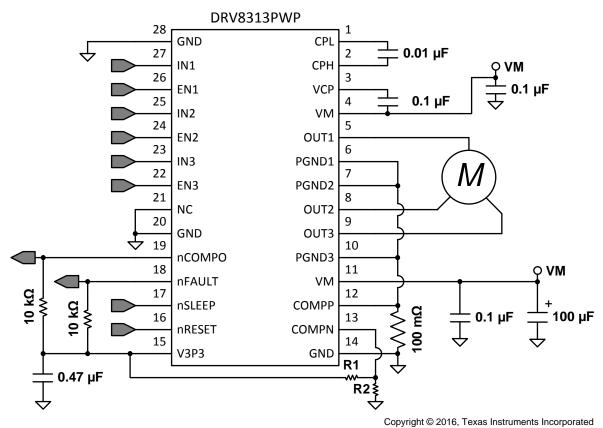
Figure 15. Uncommitted Comparator Used As a Current Monitor
