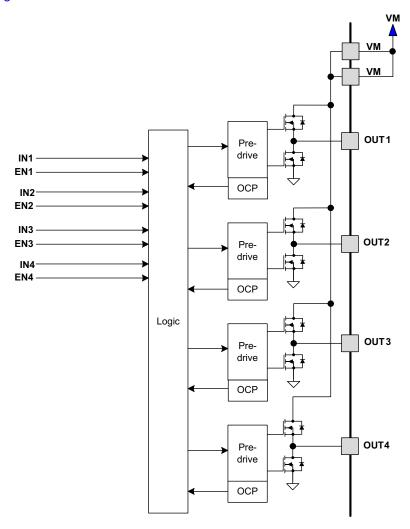
**Figure 5. Motor Control Circuitry**
