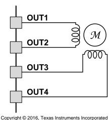
Figure 8. Stepper Motor Connections
