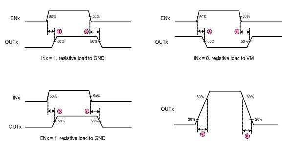
Figure 1. DRV8844 Switching Characteristics
