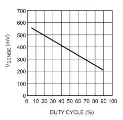
Figure 3—V<sub>SENSE</sub> vs Duty Cycle
