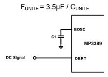
Figure 5—DC input PWM Dimming
