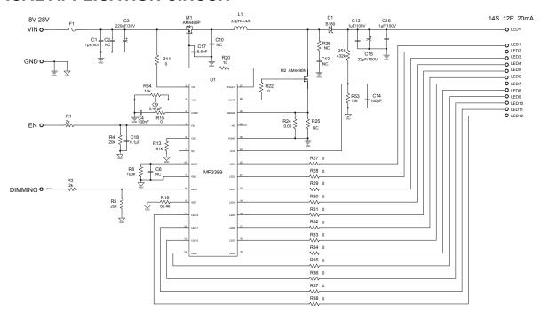
Figure 7—Drive 14 LEDs in Series, 12 Strings 20mA/string for Monitor Backlighting
