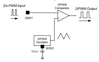
Figure 2—PWM Dimming Method
