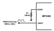
Figure 4—Direct PWM Dimming
