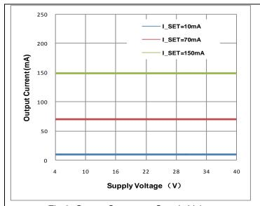
Fig 2. Output Current vs Supply Voltage
