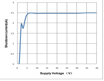
Fig 7. Shutdown Current vs Supply Voltage
