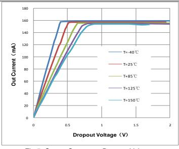
Fig 5. Output Current vs Dropout Voltage
