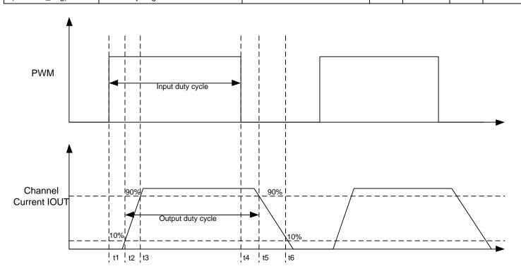
Fig 1. Output Timing Diagram
