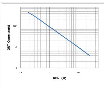
Fig 3. Output Current vs Current-Sense Resistor
