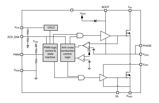
Fig. 3 - SiC634 Functional Block Diagram
