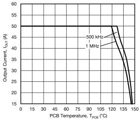
Fig. 9 - Safe Operating Area (V<sub>IN</sub> = 12.6 V)
