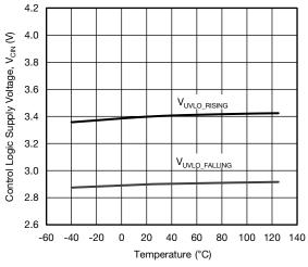
Fig. 12 - UVLO Threshold vs. Temperature
