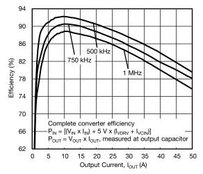
Fig. 6 - Efficiency vs. Output Current (V<sub>IN</sub> = 12.6 V)
