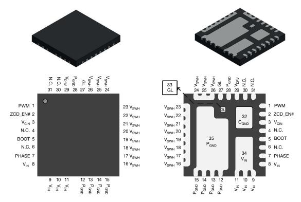
Fig. 2 - SiC634 Pin Configuration
