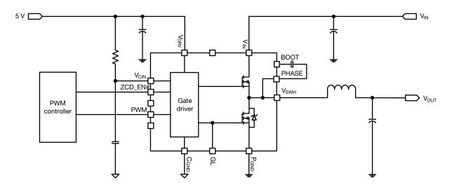
Fig. 1 - SiC634 Typical Application Diagram
