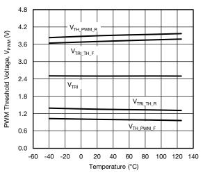
Fig. 13 - PWM Threshold vs. Temperature
