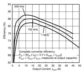
Fig. 11 - Efficiency vs. Output Current (V<sub>IN</sub> = 19 V)
