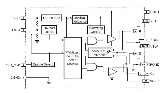
Figure 2. Block Diagram
