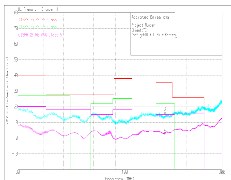
Figure 10-38. Radiated EMI Bicon Horizontal versus CISPR25 Limits
