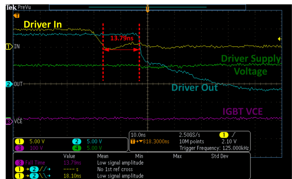
Figure 8-3. UCC27524A-Q1 Used to Drive IGBT in the Boost Converter
