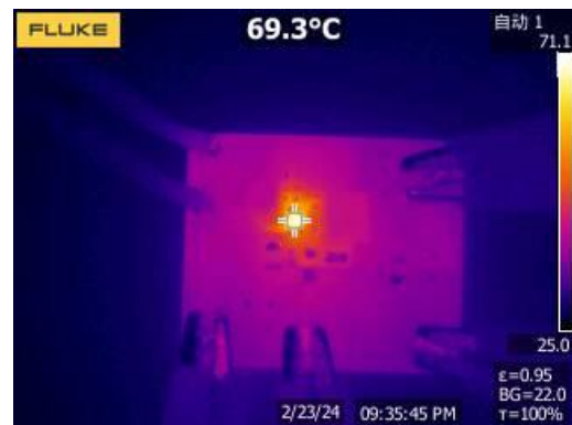
Figure 29. Thermal, 24VIN, 5VOUT, 0.8A
