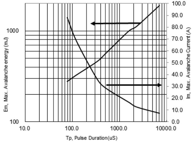
Figure 8: Single pulse Max. Avalanche Energy and Current
