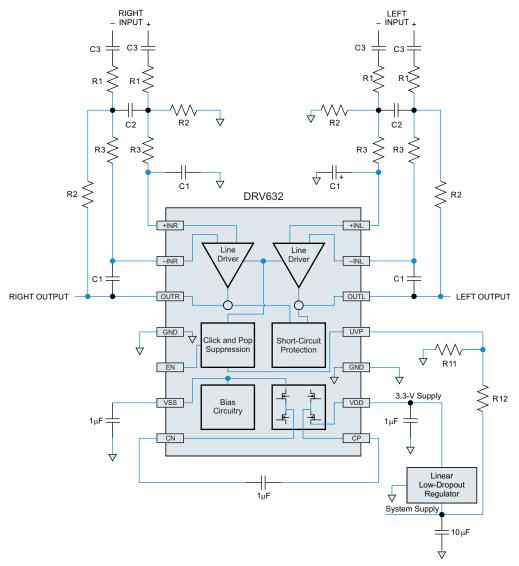
R1 = 15 k $\Omega$ , R2 = 30 k $\Omega$ , R3 = 43 k $\Omega$ , C1 = 47 pF, C2 = 180 pF Differential-input, single-ended output, second-order filter
