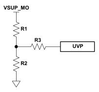
Figure 7. UVP Resistor Divider
