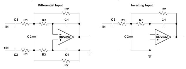
Figure 8. Second-Order Active Low-Pass Filter
