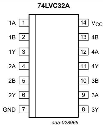
Fig. 4. Pin configuration SOT108-1 (SO14)
