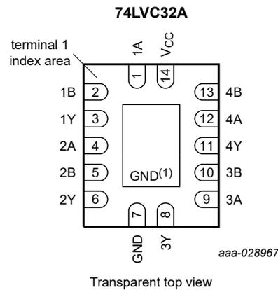
(1) This is not a ground pin. There is no electrical or mechanical requirement to solder the pad. In case soldered, the solder land should remain floating or connected to GND.
