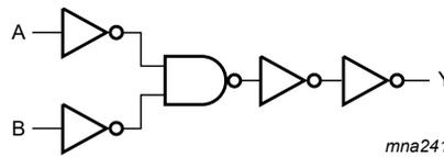
Fig. 3. Logic diagram for one gate
