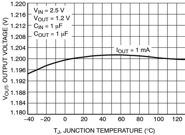
**Figure 3. Output Voltage vs. Temperature –  $V_{OUT} = 1.2\text{ V}$**
