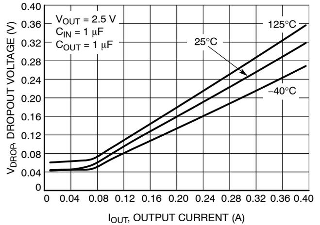
**Figure 10. Dropout Voltage vs. Output Current -  $V_{OUT} = 2.5 V$**
