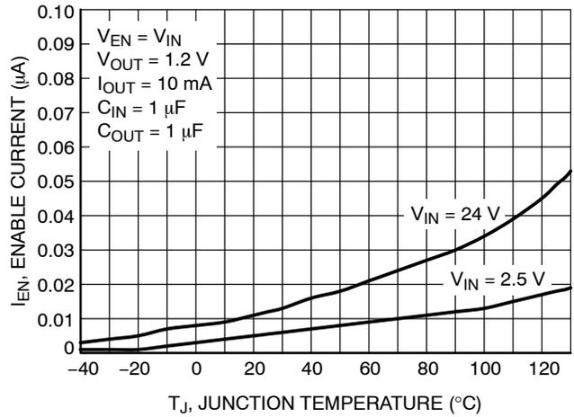
**Figure 6. Current to Enable Pin vs. Temperature**
