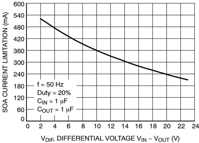
**Figure 9. SOA Current Limit vs. Differential Voltage**
