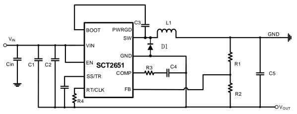
Figure 12. SCT2651 Inverting Power Supply
