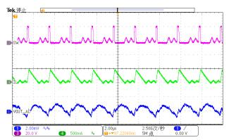
Figure 22. Output Ripple (Iload=100mA)
