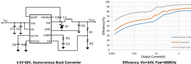
Efficiency, Vin=24V, Fsw=500KHz
