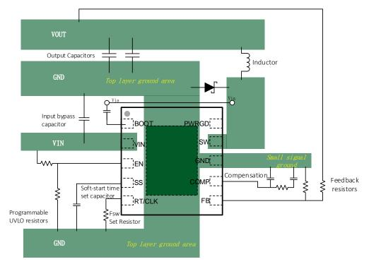
Figure 25. PCB Layout Example
