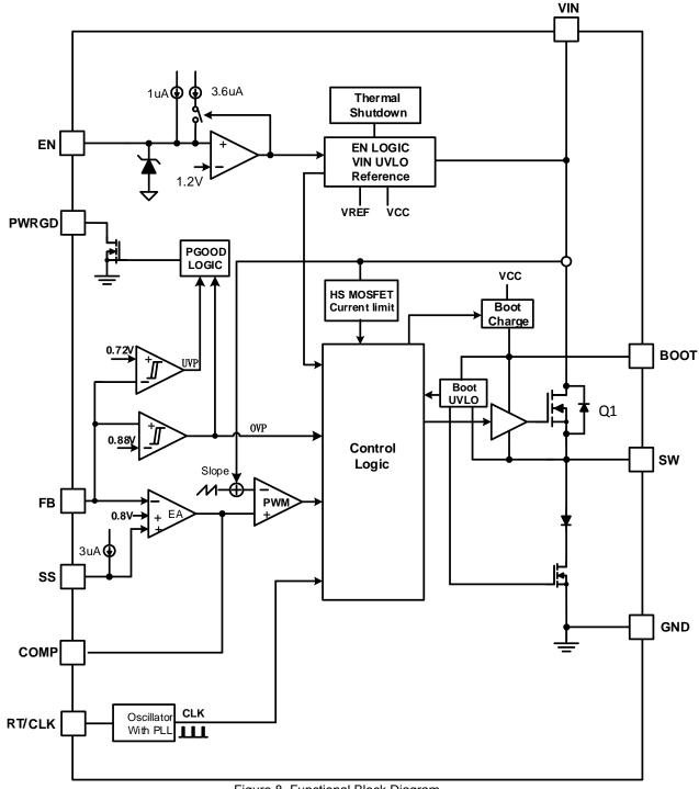
Figure 8. Functional Block Diagram
