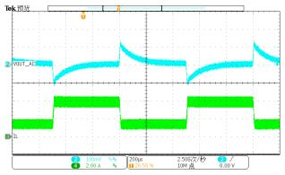
Figure 20. Load Transient (1.25A-3.75A, 1.6A/us)
