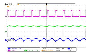
Figure 23. Output Ripple (Iload=5A)
