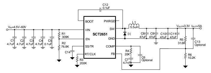
Figure 11. SCT2651 Design Example, 3.3V Output with Programmable UVLO
