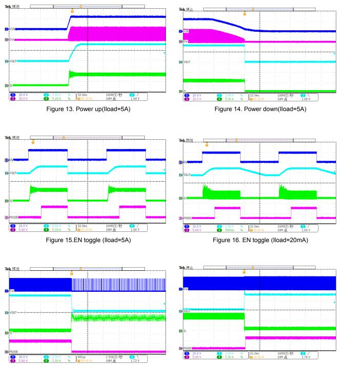
Figure 17. Over Current Protection(1A to hard short) Figur
