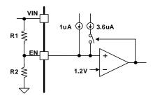
Figure 9. System UVLO by enable divide
