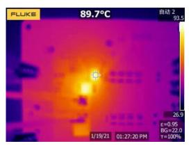
Figure 24. Thermal, 24VIN, 3.3Vout,5A
