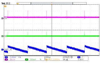
Figure 21. Output Ripple (Iload=0A)
