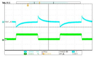
Figure 19. Load Transient (0.5A-4.5A, 1.6A/us)
