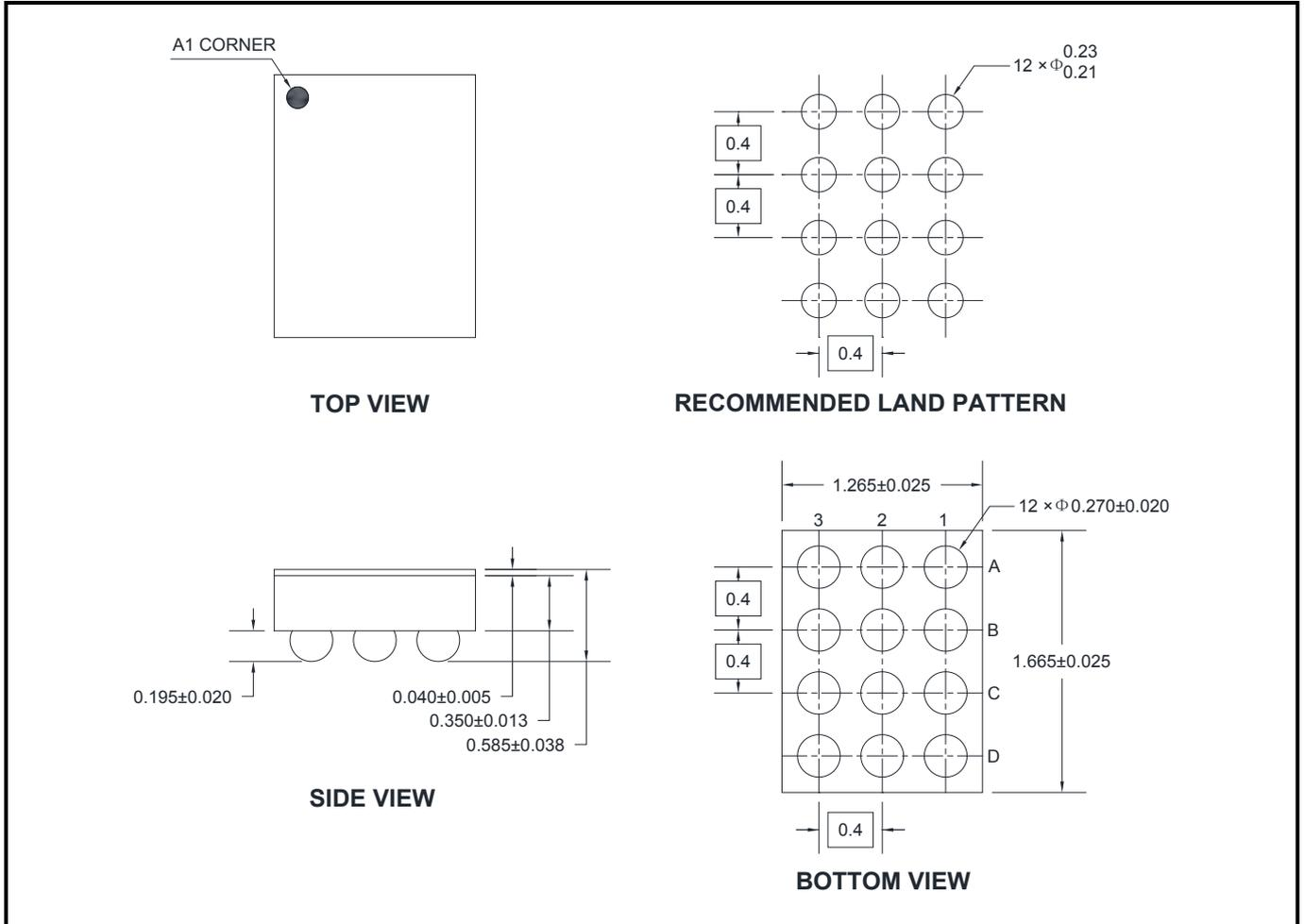
NOTE: All linear dimensions are in millimeters.
