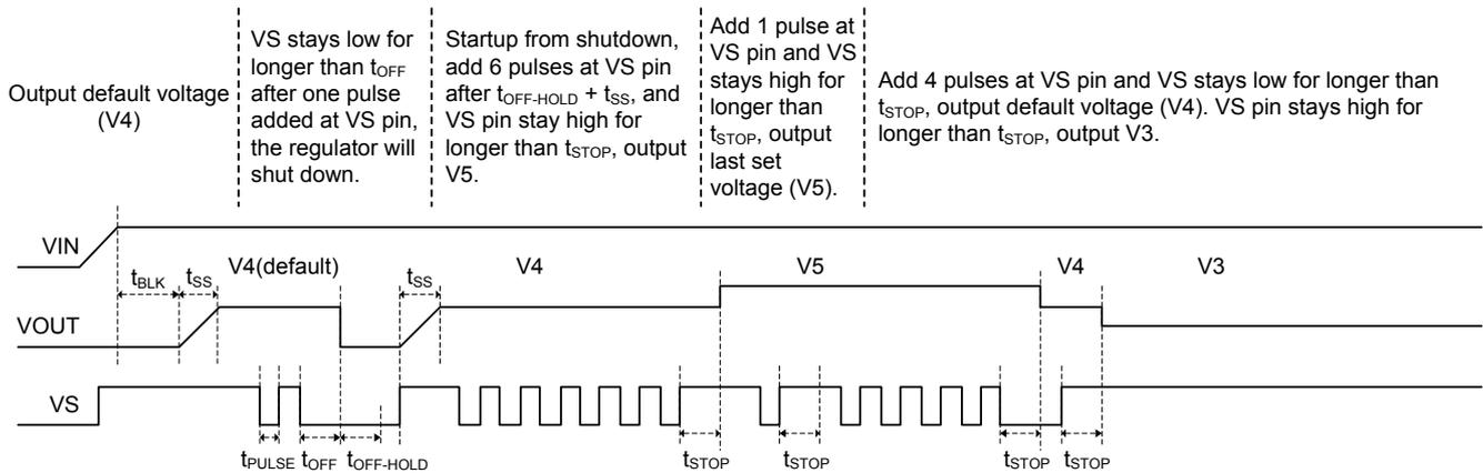
Figure 5. Program Output Voltage via VS Pin
