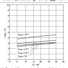
Figure 5-11. Typical Propagation Delay of High-to-Low (B to A) vs Load Capacitance T<sub>A</sub> = 25°C, V<sub>CCA</sub> = 3.3V
