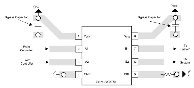
Figure 8-3. SN74LVC2T45 Layout Example
