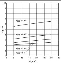
Figure 5-9. Typical Propagation Delay of High-to-Low (A to B) vs Load Capacitance T<sub>A</sub> = 25°C, V<sub>CCA</sub> = 3.3V
