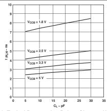
Figure 5-10. Typical Propagation Delay of Low-to-High (A to B) vs Load Capacitance T<sub>A</sub> = 25°C, V<sub>CCA</sub> = 3.3V
