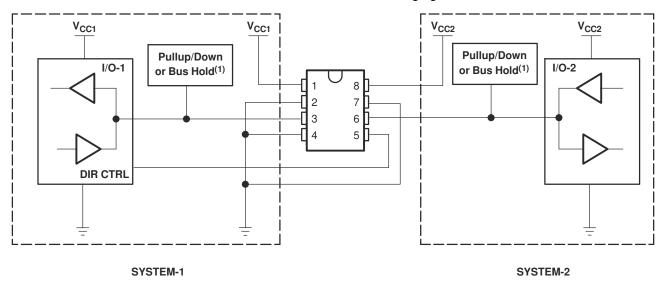
Figure 8-2. Bidirectional Logic Level-Shifting Application
