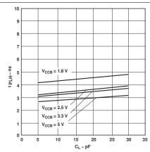
Figure 5-12. Typical Propagation Delay of Low-to-High (B to A) vs Load Capacitance  $T_A = 25$ °C,  $V_{CCA} = 3.3V$
