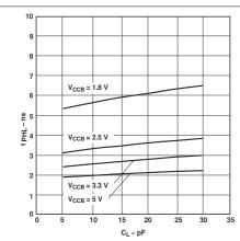
Figure 5-13. Typical Propagation Delay of High-to-Low (A to B) vs Load Capacitance  $T_A = 25^{\circ}C$ ,  $V_{CCA} = 5V$
