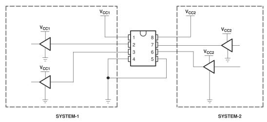
Figure 8-1. Unidirectional Logic Level-Shifting Application
