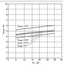
Figure 5-7. Typical Propagation Delay of High-to-Low (B to A) vs | Figure 5-8. Typical Propagation Delay of Low-to-High (B to A) vs Load Capacitance T<sub>A</sub> = 25°C, V<sub>CCA</sub> = 2.5V
