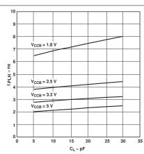
Figure 5-14. Typical Propagation Delay of Low-to-High (A to B) vs Load Capacitance  $T_A = 25^{\circ}C$ ,  $V_{CCA} = 5V$
