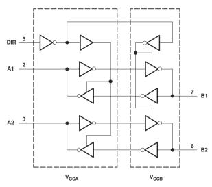
Figure 7-1. Logic Diagram (Positive Logic)
