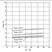
Figure 5-15. Typical Propagation Delay of High-to-Low (B to A) vs Load Capacitance T<sub>A</sub> = 25°C, V<sub>CCA</sub> = 5V
