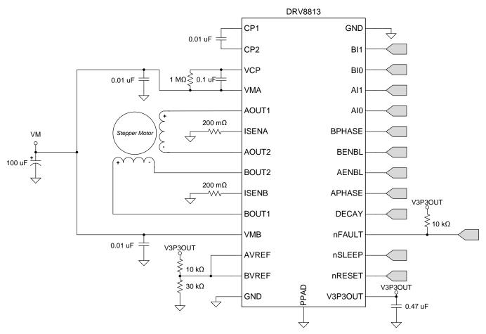
Figure 7. Typical Application Schematic
