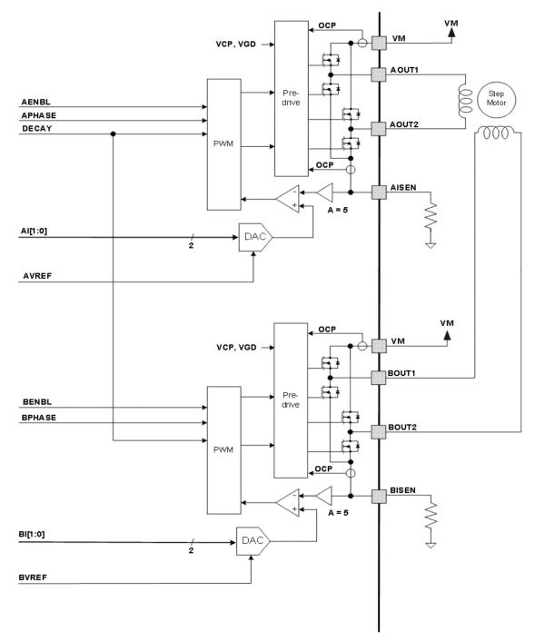
Figure 5. Motor Control Circuitry
