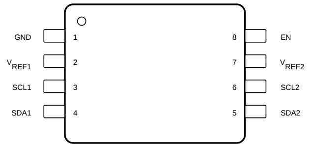
Figure 5-2. DCU Package 8-Pin VSSOP (Top View)
