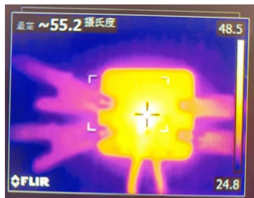
Figure 20. Thermal, 12VIN, 3.3Vout, 3A(SOT563)
