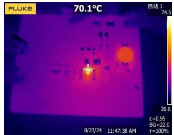
Figure 23. Thermal, 48VIN, 12Vout, 1A
