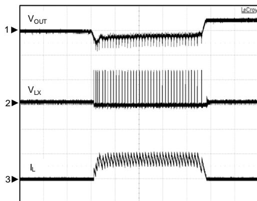
CH1:  $V_{OUT}$ , 100mV/Div, AC
