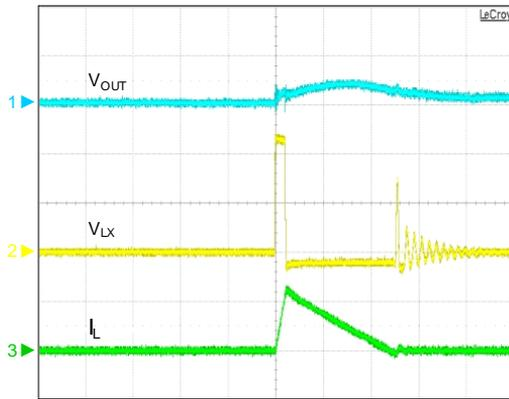
CH1:  $V_{OUT}$ , 50mV/Div, AC
