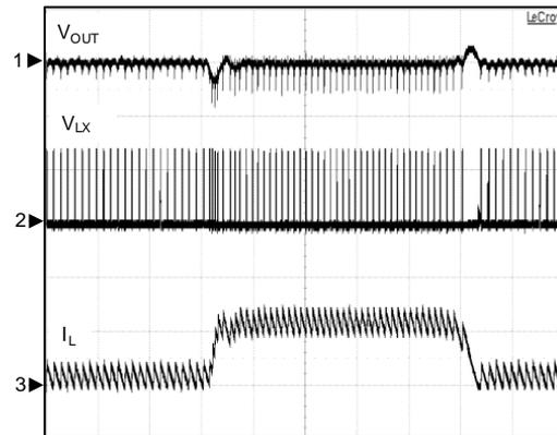
CH1:  $V_{OUT}$ , 100mV/Div, AC
