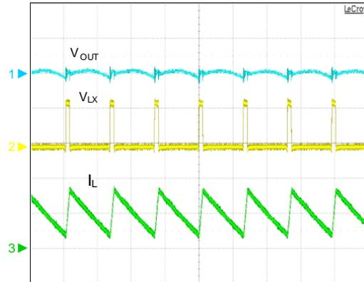
CH1:  $V_{OUT}$ , 50mV/Div, AC
